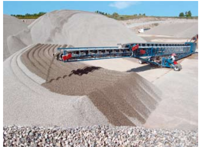
22 Mobiles teleskopierbares Haldenband (Thor Global) Mobile radial telescopic stacker (Thor Global)
