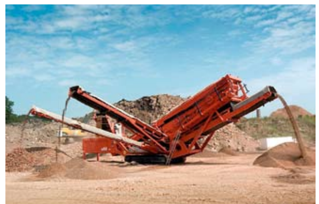
12 Raupenverfahrbares Tripledeck-Sieb (Sandvik) Triple-deck screen mounted on crawler tracks (Sandvik)
