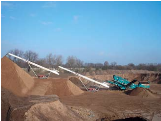
21 Telestack Haldenbänder (C. Christophel GmbH) Telestack tracked stockpiling conveyors (C. Christophel GmbH)
